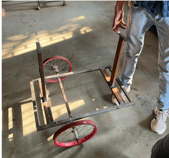
Fig 6.2 Fabrication of chassis.
