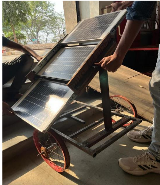
Fig 6.4 the mounting of the array on panels with bearings.
